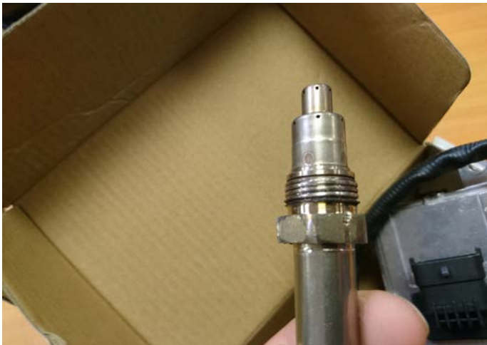
Figure 11. Damaged sensor thread and nut.
