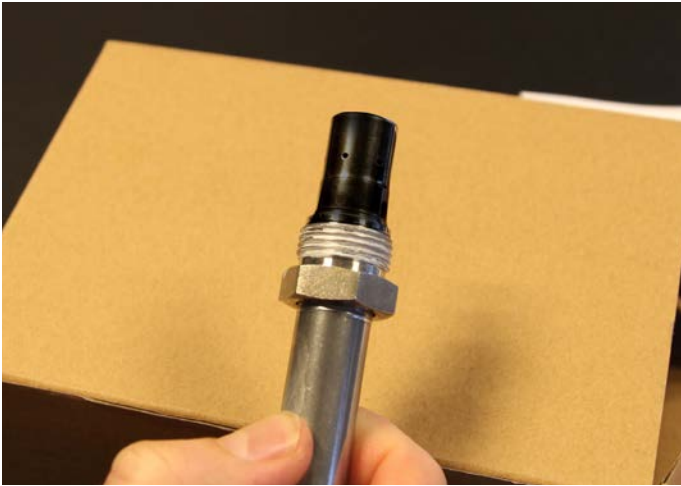
Figure 12. Evidence of excessive soot/ash.
