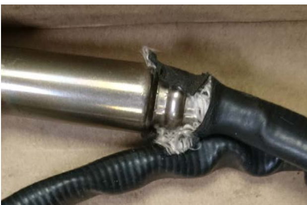
Figure 14. Evidence of damaged wiring.
